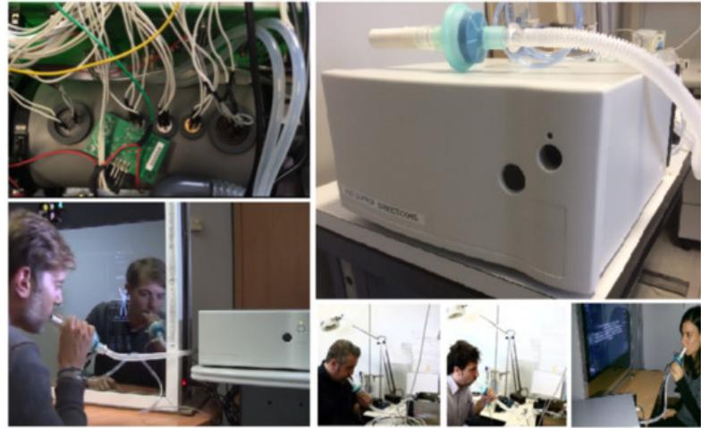
The Wize Sniffer (WS). On the top, left: the gas sensors in the gas sampling chamber are shown. On the top, right: WS external configuration. Others: the WS while performing a breath test
