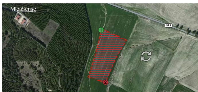
Fig. 4. (b) The flight plan for multispectral survey of the field
